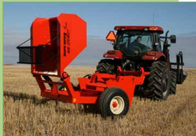
An electric solenoid lets you back up and dump with the flick of a switch from your tractor.
